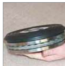
Ball bearing for turning plate
